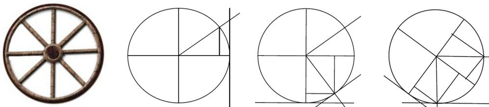
Suppose we place the wheel with the  $x$  axis touching the ground and then roll it to the right a distance of half a quarter of a turn. (See figure above on the right.) The center of the wheel moves forward parallel to the ground at a constant velocity as the wheel turns. The direction of center point motion is thus always parallel to the tangent line of
