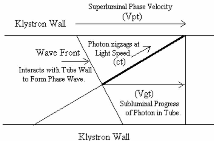
The klystron wave guide used in microwave technology clearly shows the relationships of the three wave types.  $(V_g)$  is the group velocity,  $(V_p)$  is the phase velocity, and  $(c)$  is the photon moving at the speed of light. We convert velocities into relative distances by multiplying each velocity by the same unit of time ( $t$ ) which then cancels out of the equation.
